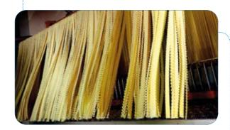
Rapid drying at high temperatures is a technology that results in huge time-savings and, with alternating drying and resting stages having practically disappeared, drying times are down to an average of 4-6 hours for long shape pasta and 3-5 hours for short shape varieties.
